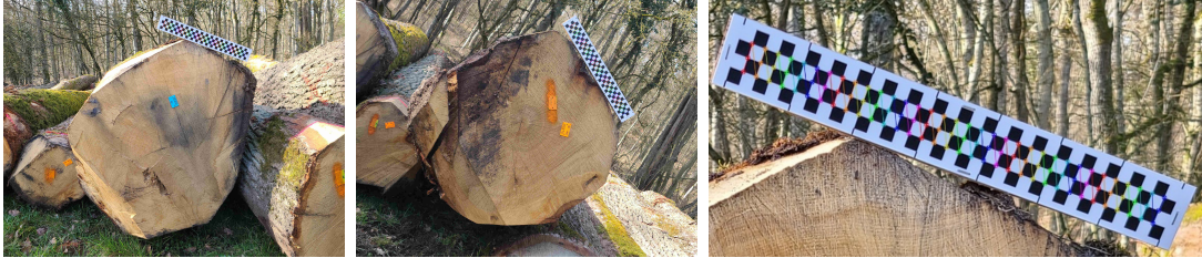
Figure 1: Photos taken at the bottom end of oak logs. A black and white checkerboard pattern is placed on the log so that size information can be retrieved. Here, an OpenCV function enables to automatically detect this checkerboard pattern (on the right).
